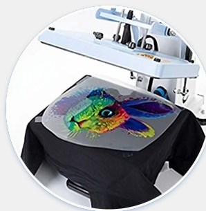
5. Press on garment at 150°C / 20 seconds, using a firm pressure.
